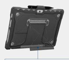
Smooth friction-hinge kickstand delivers unlimited positioning
